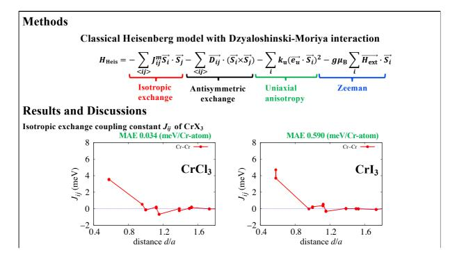
We use classical Heissenberg model with isotropic exchange, antisymmetric exchange or DMI, uniaxial anisotropy, and Zeeman term. All parameters of Monte Carlo simulations are obtained from first principles calculations.
