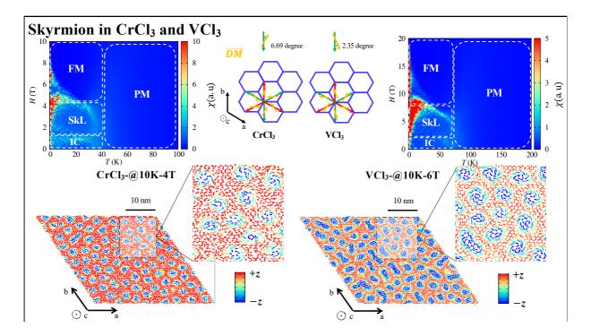
We also found that VCI3 also have similar magnetic phase diagram as CrCl3. However, the DM vector of VCl3 is nearly opposite with CrCl3. It leads to two type of skyrmion with diferent helicity. If we can control the electron or hole dope in multilayer, we might control the helicity of the materials. Note that the skyrmion diameter is quite small, about 2 nm due to the centrosymmetric materials.
