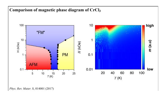
Then we calculate the magnetic phase diagram of CrCl3. the blue color means magnetization is small, it is AFM or PM in experimental phase diagram. The red color means the magnetization is high, it is FM in experimental. Here at this temperature, the red region is expand in low magnetic field region. We got a good agreement with experimetal study.
