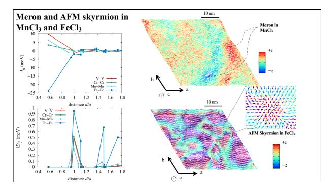
We also found the Meron in MnCl3 and AFM skyrmion in FeCl3. In MnCl3, the magnetic anisotropy is easy plane with ab plane, it leads to the formation of Meron at zero external magnetic field.
