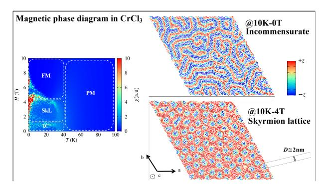
Then we check the snapshot of Monte Carlo simulations for making the magnetic phase diagram in magnetic susceptibility. At 10 K and 0 T, the magnetic phase is incomensurate with broken of long range order. If we apply magnetic field like 4 T, we can get the skyrmion lattice in CrCl3.
