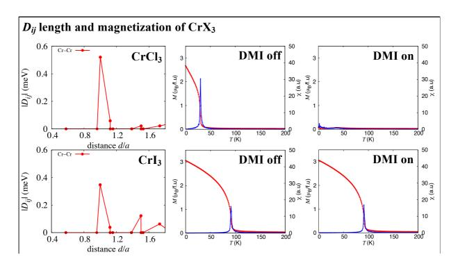
Then we consider the DMI in first principles calculations. The DMI of second nerest neighbor of intralayer is finite and quite large even in CrCl3. As point out in previous slide, the results of MAE and Jij in CrCl3 does not suport the inplane AFM in experimental works. And if we calculated the magnetization with switch off DMI, all CrX3 shows clear FM-PM transition with the ground state being FM.
