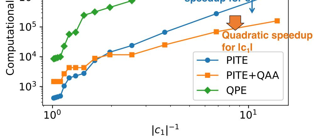
Computational cost was estimated when the infidelity was below  $\delta = 10^{-4}$ . QAA is efficient for  $lc_1 l < 1/2$  due to overhead of QAA.
